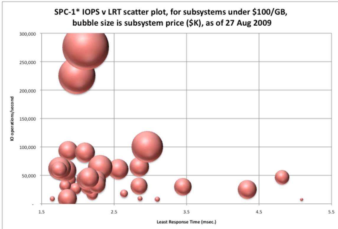
**Figure 3 SPC-1 Bubble chart of IOPS against LRT, bubble size proportional to subsystem price**
